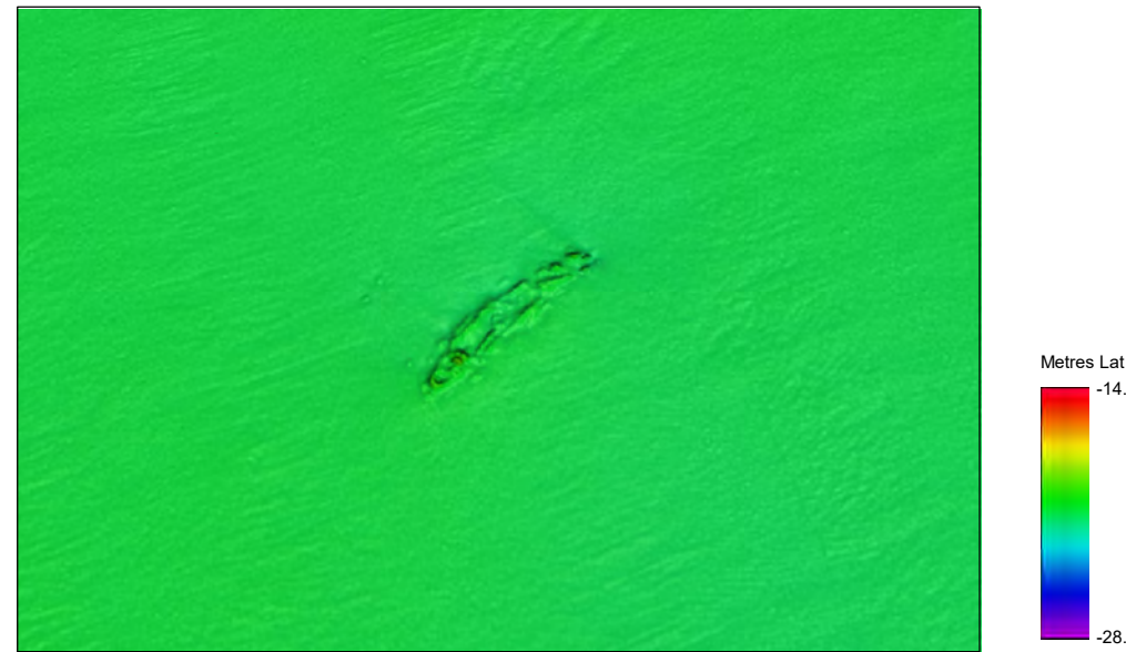
Multibeam bathymetry image of 72574 looking looking south-south-east (x1 vertical exaggeration)
