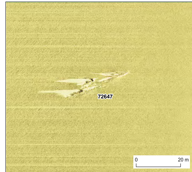
Sidescan sonar image looking north-east of 72647 , measuring 45.2 x 20.3 x 2.4 m
