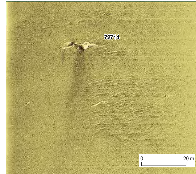
Sidescan sonar image looking south-east of 72714 , measuring 20.1 x 14.6 x 1.7 m
